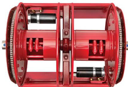
Chain & sprocket drive powered by 2 electric gear motors
